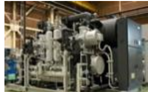
High-efficiency refrigerator, Mayekawa MFG, Indonesia
